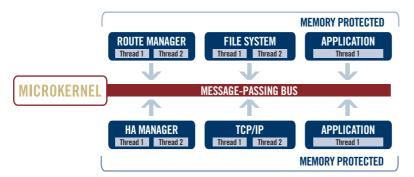
Operating systems that contain a number of cooperating components, such as the QNX Neutrino microkernel RTOS, use separate processes to run system services. Performance can increase due to the number of independent components that can operate concurrently in multiprocessor CPU configurations.
