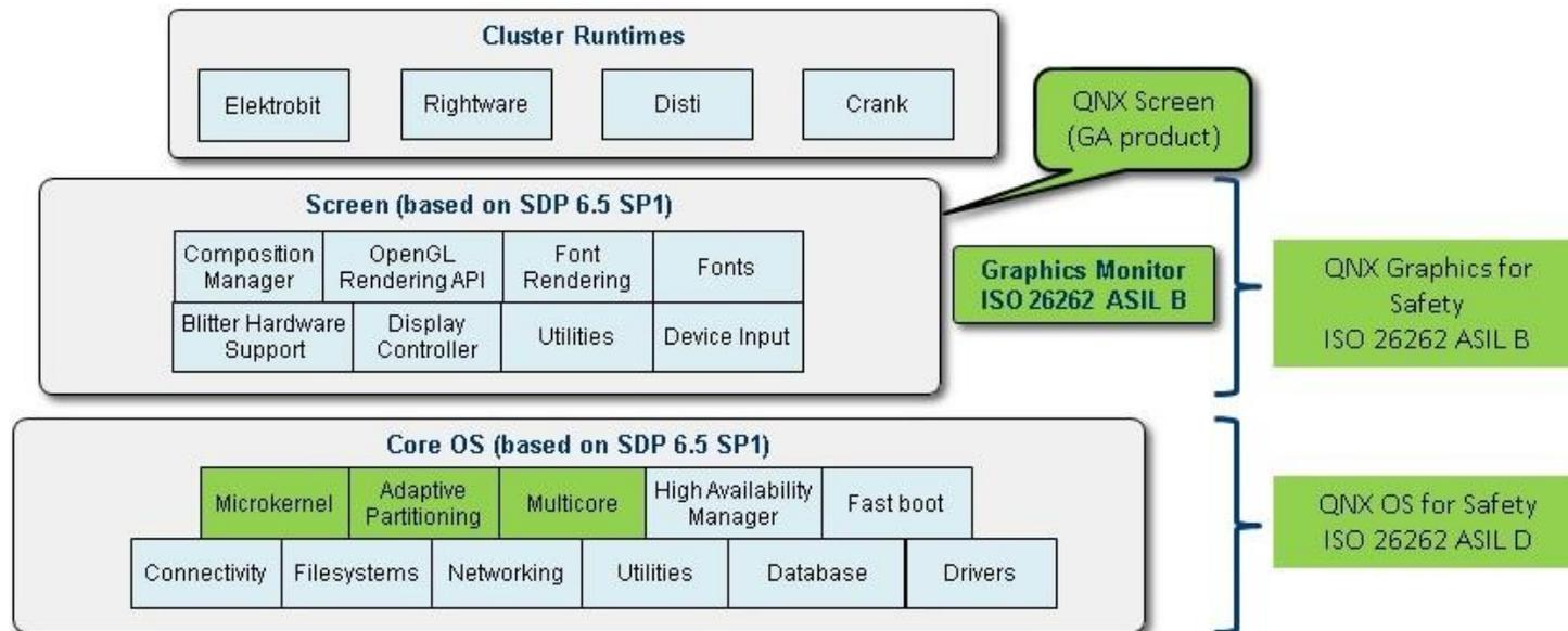
The figure above illustrates the various component required to form a typical digital instrument cluster and the fit of QPIC 1.0 in the context.
