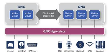
Figure 1: When both guest OSs are QNX, patented technology is used to share devices without the need to write custom drivers.
