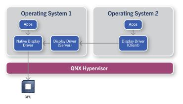
Figure 2: QNX technology allows GPU devices to be shared by guest OSs so each can render graphical output to external displays.
